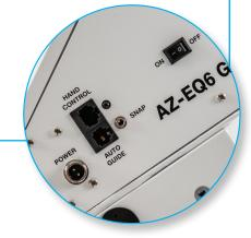
• We came across a minor quirk when polar aligning the mount. If you power it up and then rotate the dec. axis so that you can view and align Polaris through the polarscope, you also activate the dual encoders. On successive attempts we found the scope always pointed 90° away from the first alignment star. We found that it was better to do the polar alignment, turn the power off and line up the scope north, then power back up again. After doing this we could align every time.
